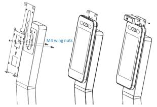
The figure below shows the process of installing the digital temperature measurement module on a standing pole when the module is to be used in combination with a face recognition terminal.
